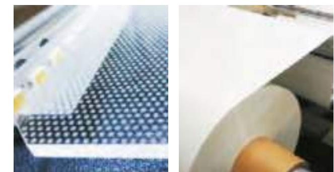
Glowes are true PMMA material, pure clear, transparent, transmittance above 93%. After Laser Dotted, this plate is optimal for light transmission. The LGP, commonly, work with a Reflector & Diffuser, to transfer the light from the edge to the top. These three, or in some case, two of them plus LED Engine make up a background lighting system.
